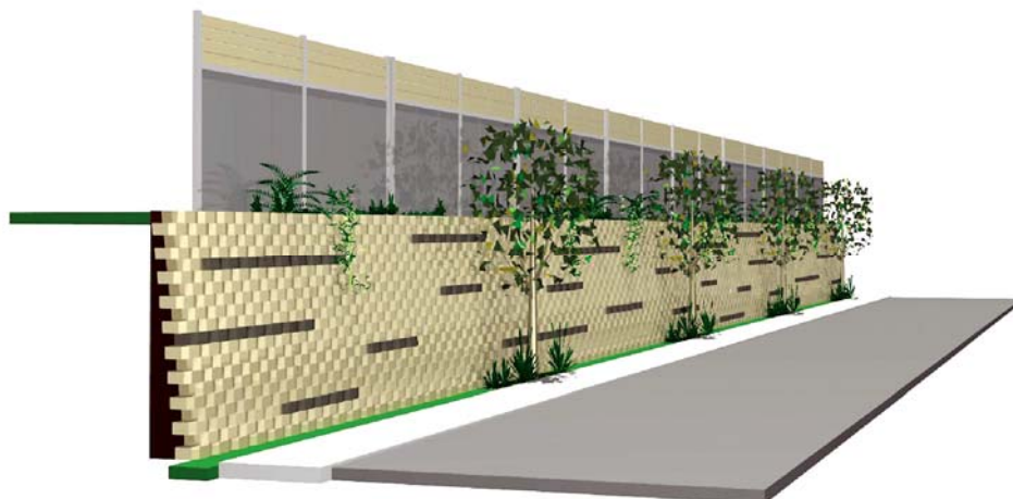
Figure 5.6 Refined concept design of retaining structure and noise barrier at Broomfield Street
